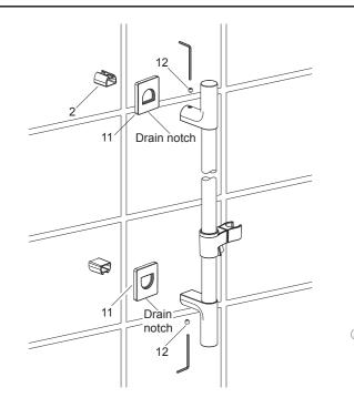
Slide the bracket escutcheons(11) onto the bases(2), confirm the drain notch of the escutcheon is pointed down. Install the whole slide bar onto the bases.
